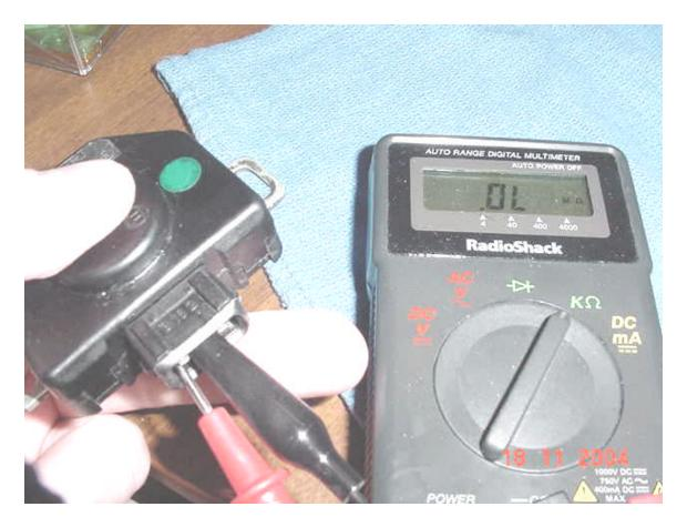
This should not show continuity ("OL" on meter signals infinite resistance).
