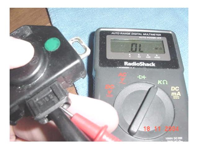
This correctly shows discontinuity of the idle circuit at this point.
