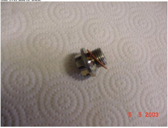
Thread this into the oil pan by hand then torque sequentially (couldn't find torque value in any of the manuals so I used 25 ft-lbs). <u>Don't guesstimate – use a torque wrench.</u> Stripping the oil pan threads would make this much more interesting.
