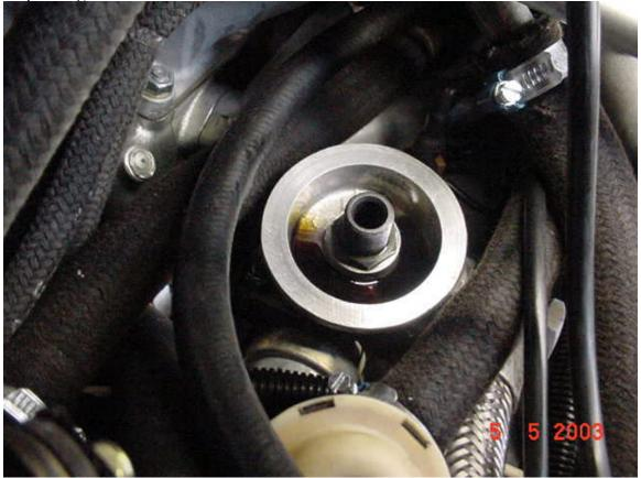
Wipe a bit of oil on the new filter rubber seal and install hand-tight. Tighten further using the filter wrench; I protected the nice white paint by covering the UFI filter with a Ziploc freezer baggie & lining inside of the filter wrench with masking tape. Not certain about a
