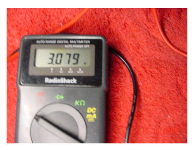
Tachometer signal: (-) lead on #11 and (+) on #24. Normal output is 0.2-0.35v.
