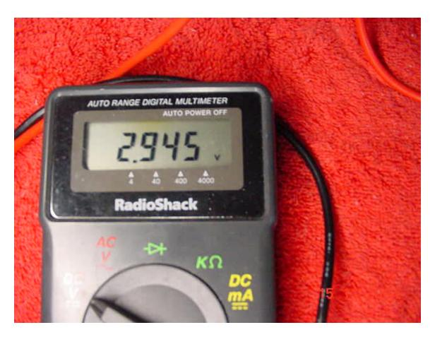
ECU output signal to 1-4 bank coil: (-) lead on #15 and (+) on #14. Normal is 2.8-3.5v. If no output, ECU is faulty.
