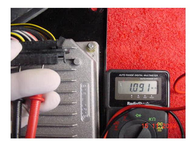
Turn the key to "run" (not start). Check for input voltage by setting meter to DC with (-) lead on #11 and (+) on #13. Normal is 11-13v (meter reads 11.6v)
