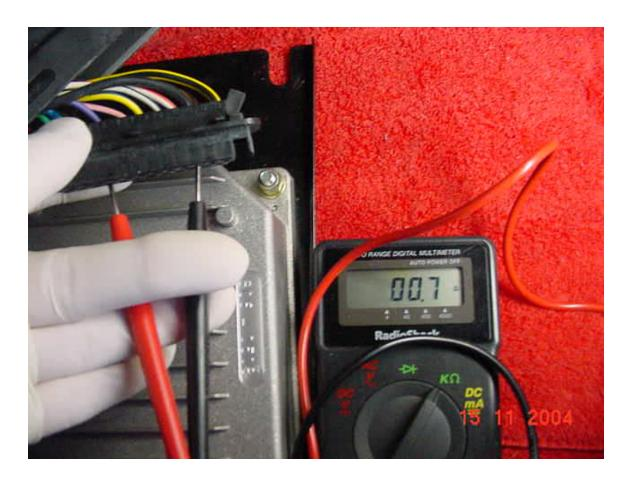
The manual then lists #11-#18 & #11-#23 for "advance curve identification as having infinite resistance. They must, since my connector didn't have wire inputs to either #18 or #23.
