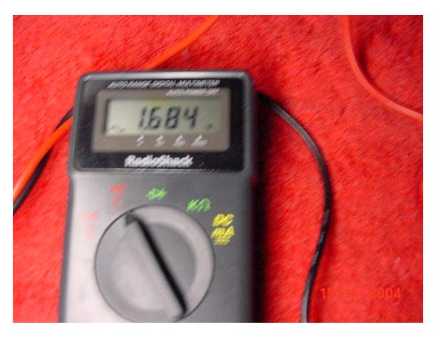
ECU output signal to 5-8 bank coil: (-) lead on #10 and (+) on #9. Normal is 2.8-3.5v. If no output, ECU is faulty.
