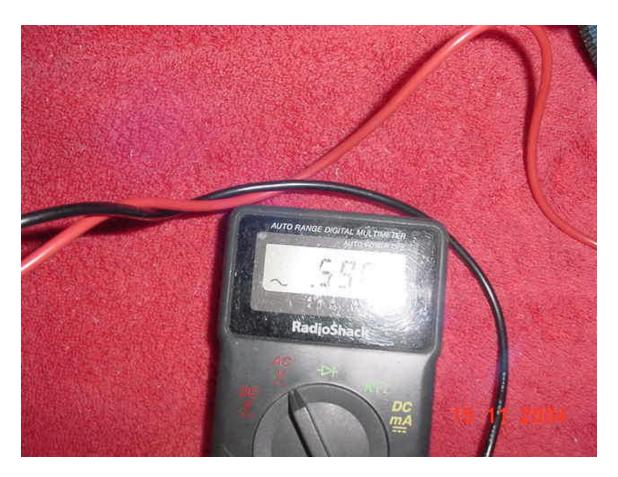
• RPM sensor AC voltage: (-) lead on #3 and (+) on #16. Should read >2.0v.
