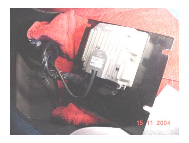
Remove the main ECU multi-terminal connector. Remove the small screw on top and gently slide the rubber boot back. Two more screws are exposed at the base. Remove both and the back reinforcement plate lifts off. The multi-connector is then maneuvered out of the cover:
