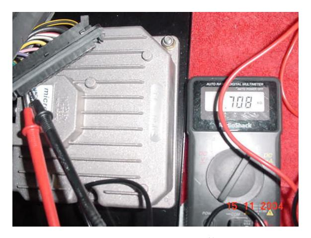
• RPM sensor resistance: #3-#16: 600-1000ohms (if 0 ohms or >1500ohms abnormal)
