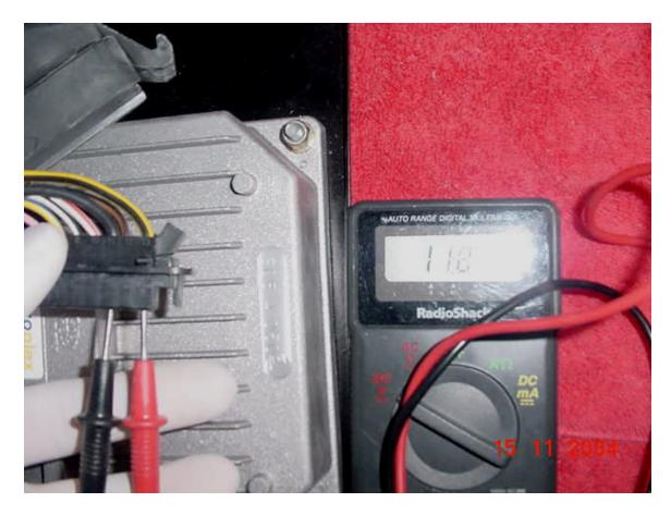
Reconnect the multi-terminal to the ECU, leaving cover off so wire terminals can be back-probed. Start the car and allow to warm. At idle, measure the following:
