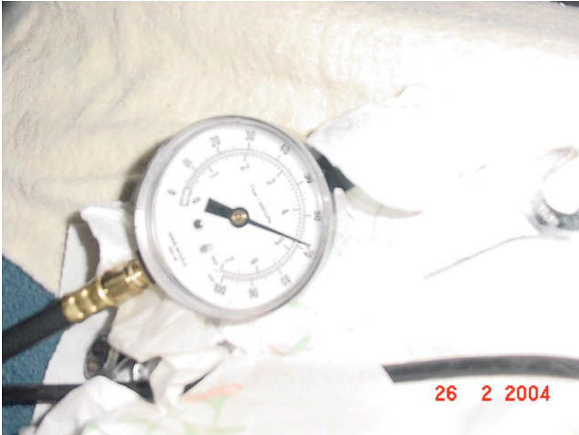
Turn ignition off. Pressure will rapidly fall to approximately 40psi and hold. Allow car to stand for 20 minutes; the accumulator should hold a minimum of 3-3.5 bar (approximately 40psi) for minimum 10-20 minutes if functioning properly and injectors are not leaking.
