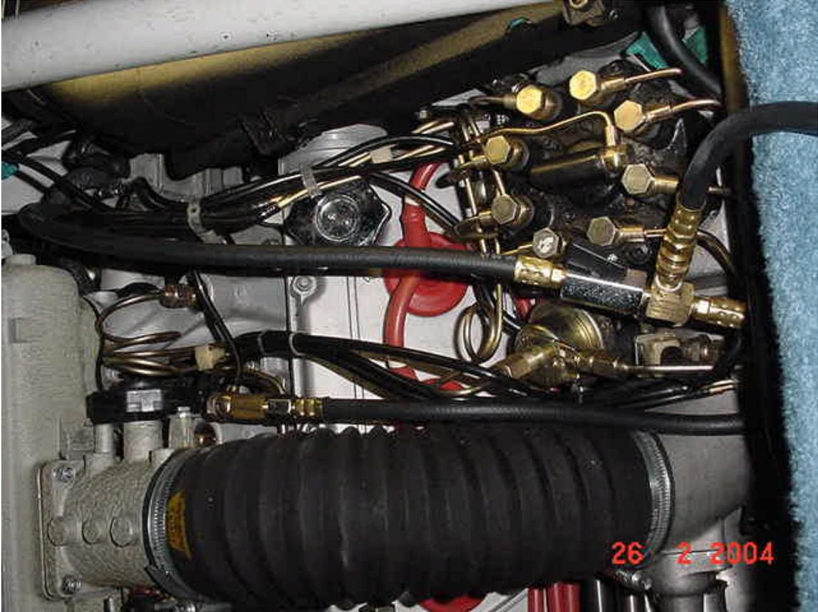
Remove the blue fuel distributor safety switch connection from the rear of the mixture control unit to allow the fuel pump to run without actually starting the engine. I also disconnected the cold-start injector in case it was signaled, but this is probably unnecessary. Temporarily disconnect the input signal harness to the WUR:
