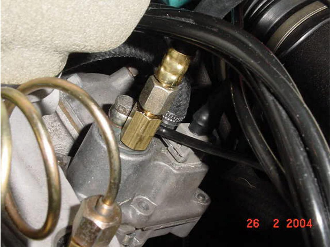
My pressure gauge line then attached to the T-fitting using a snap-collar type lock:
